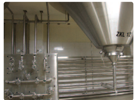
Typical arrangements in the cellar below conical FVs. Pipe fences in use at Ulm in Germany and Pottsville in the USA.
