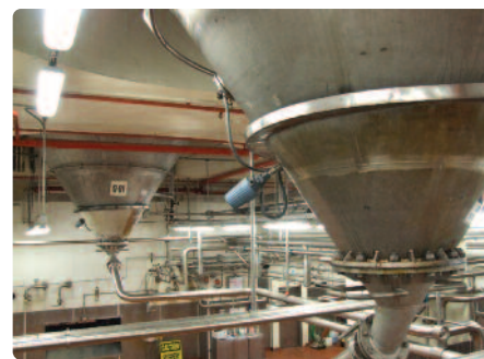
D cellar at Fosters in Melbourne, the home of 6600hl 7-metre diameter monster vessels.
